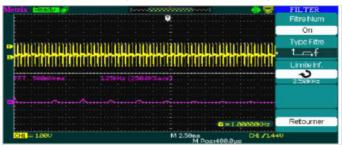
If you apply a low pass filter with a cut-off frequency Fc=2.5 kHz, the harmonics of the 1 kHz calibration signal are attenuated
