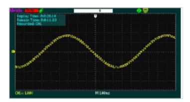
**In Recorder mode**, it is not possible to zoom after acquisition. The segments have a constant depth of 2,500 points and, for each frame, all the points are shown on the screen, i.e. 2,500/18=138 points per division.
