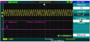
If you apply a band stop filter with a low cut-off frequency Fclow=2.5 kHz and a high cut-off frequency Fchigh =5 kHz, you will attenuate harmonic 2 of the 1 kHz signal:
