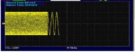
Caution: to switch automatically to "SCAN mode" by turning the "S/div" button, you must be in "Auto" trigger mode. If the trigger is in Normal mode, it is impossible to switch to "SCAN mode":
