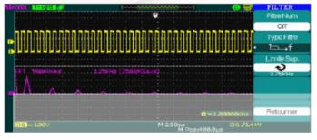
If you apply a high pass filter with a cut-off frequency Fc=2.5 kHz, the fundamental of the 1 kHz signal is attenuated, while leaving the harmonics:
