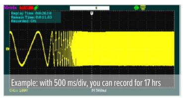
After stopping the recordings and selecting a recording (acquisition in Min/Max mode with Normal or Long Mem memory depth), you can zoom down to 1 ms/div, i.e. a maximum zoom factor of x500
