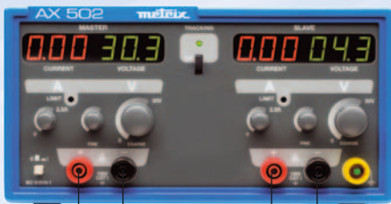
Mounting in series: 60 V - 0 to 3 A
