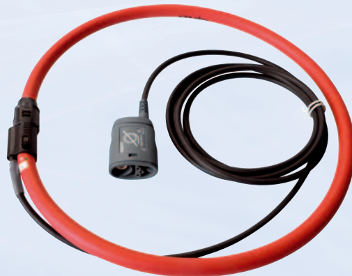
HX0072 AmpFLEX™ current sensor 5 A - 3 000 Arms / 200 kHz
