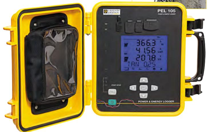
To improve **energy efficiency according to ISO 50001** or carry out the audits required by the regulations, the PEL 105 can be set up on the different electrical feeders. It can then be used, simply and without downtime, to assess the relative weight of each line as a proportion of overall consumption, define a load profile for the installation and thus determine the priorities for improvement.
