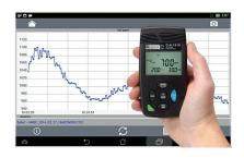
to select the type of lighting they are monitoring, with built in spectral and incidence correction, and display the measurement in Lux, as well as providing mapping functionality to ensure adequate lighting coverage throughout the facility. From an energy efficiency point of view, light level mapping is also important to ensure no particular area is over lit.
