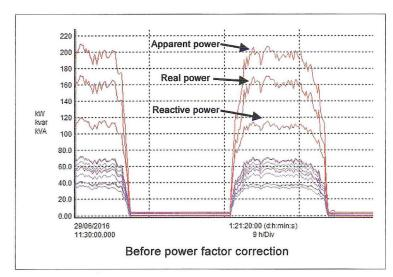
factor is a ratio of the real power that is used to do work and the apparent power that is supplied to the circuit.
