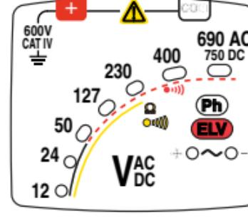
If there is a perturbing voltage near the element being tested, the device may indicate the presence of an operating voltage on the element being tested.
