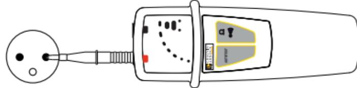
If the test probe is in fact on the phase, the **Ph** (phase) indicator flashes and the device beeps.
