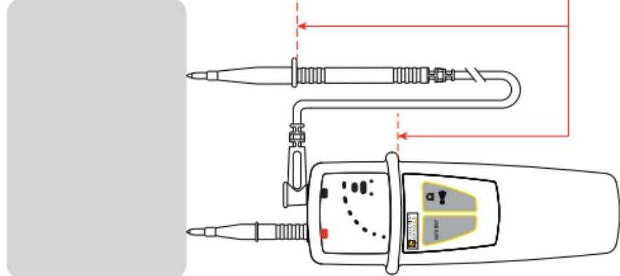
Place the test probes on the element to be tested and maintain a firm contact.
