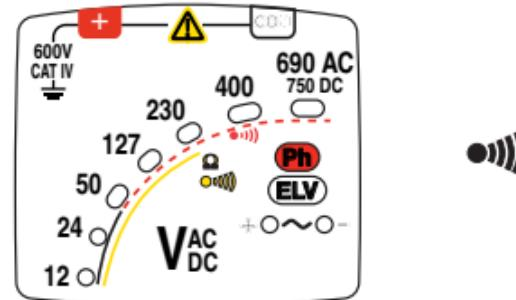
**Warning:** if the **Ph** indicator is not flashing, that does not mean that there is no hazardous voltage on the outlet.
