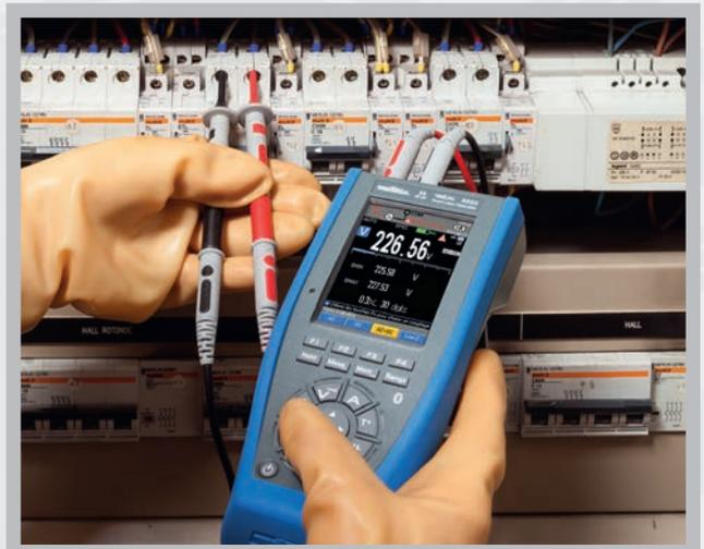
Measurements on electrical cabinets
