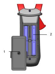
Figure 6: the battery compartment cover
