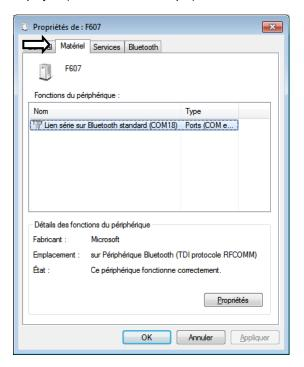
2.3 Device connexion in progress with PAT software, with Bluetooth. Choose only « Port COM » to communicate, and choose the good port COM (COM18 here)
