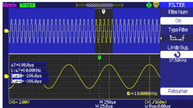
We are now going to observe the effect to the “Low-Pass” filter on the 10 kHz/80 kHz sine wave using the FFT.
