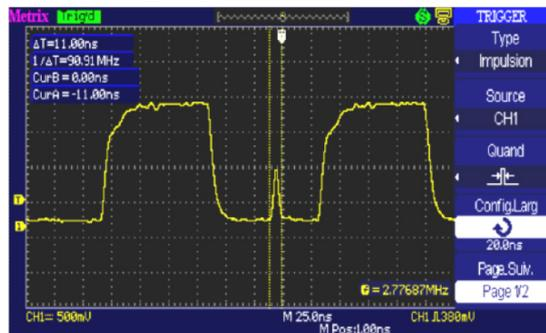
Use the Delayed and LongMem mode in order to be able to analyse the fault and the digital frame in detail.
