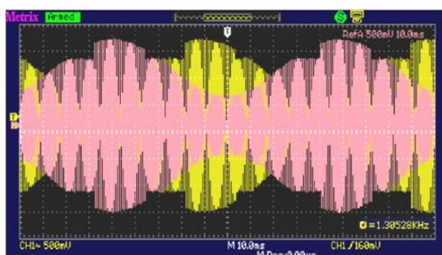
We can press the “REF” key to record the signal on one of the 2 channels as reference, then validate this reference by “On” and observe the variations of the real-time signal of the channel with respect to the frozen reference.
