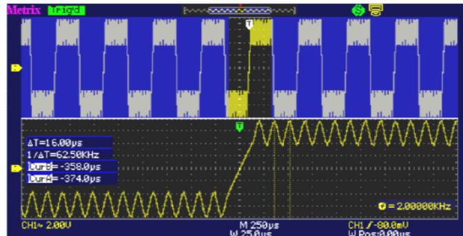
b) A "low-pass" digital filter having a high cut-off frequency of 25 kHz is applied to this signal:
