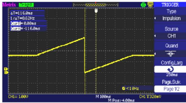
By placing the triggering level above the mean level of the signal and acting on the width of the positive pulse, it is possible to synchronise to the high pulse.
