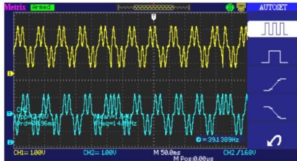
When Autoset is exited, the oscilloscope adjusts the vertical position so that the traces are not superposed.
