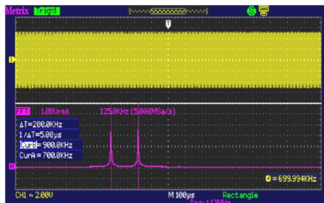
Using a bandpass filter centred on  $700 \text{ kHz}$ , then on  $900 \text{ kHz}$ , we are going to be able to isolate these 2 spectral components.
