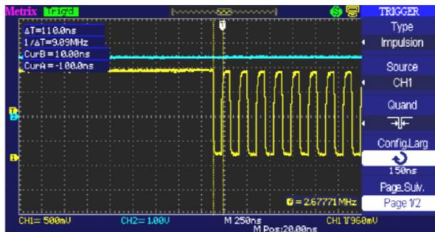
Set the triggering to pulse width < 20 ns and adjust the triggering level to close to the low level of the pulse in order to trigger on the fault.
