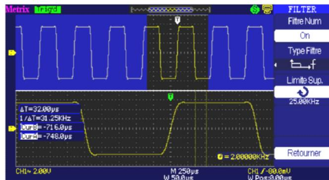
c) A "high-pass" digital filter having a low cut-off frequency of 25 kHz is applied:
