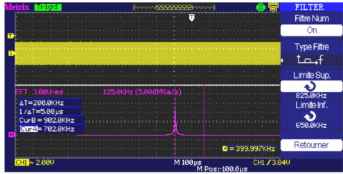
Display of the 700 kHz spectral component with delayed time base.
