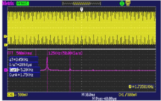
The "Voltage" cursors can be used to determine the amplitude of the harmonics:
