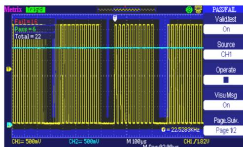
The Pass/Fail function displays the number of times that the signal has satisfied ("Pass") or not satisfied ("Fail") the mask defined.
