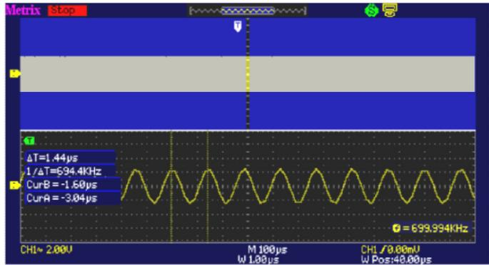
b) A bandpass filter (825 kHz, 1 MHz) is used to isolated the 900 kHz component:
