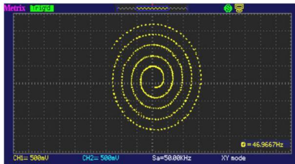
The geometrical shape obtained in XY depends on the sampling rate, which in our example is  $F_{\text{sample}} = 50\text{ kHz}$ .
