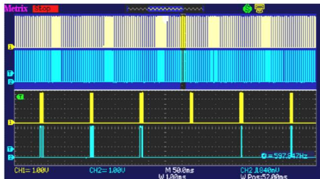
The proposed signal is representative of a communication bus with “data - 8 bits” and a clock.
