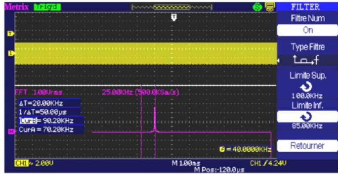
We view the filtered signal and use the cursors to measure its frequency,  $F = 90$  kHz, and its amplitude = 5.12 V peak to peak:
