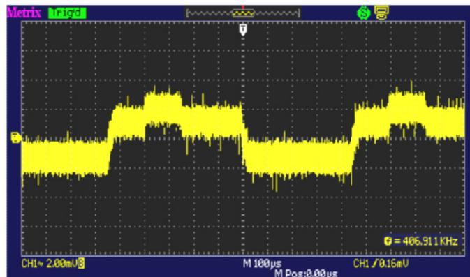
b) The use of a 100 kHz digital low-pass filter makes it possible to analyse the signal without the noise.
