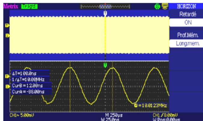
But when the memory depth is “Normal”, the 10 MHz sinusoidal signal is no longer properly reconstituted, because the 400 ns sampling interval is longer than the 100 ns period of the 10 MHz sinusoidal signal:
