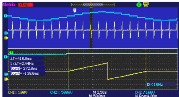
c) The measurements can be made using the manual cursors, but it is also possible to display the 23 automatic measurements made on the desired channel simultaneously.
