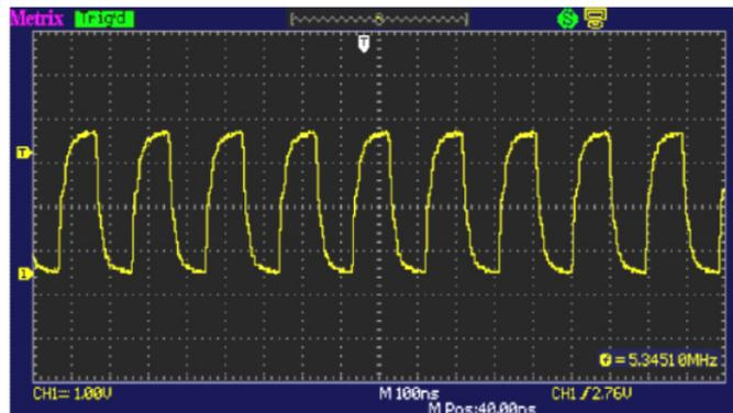
c) Enter Delayed mode with 10 ns/div. for the delayed time base.
