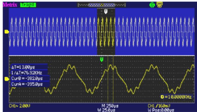
When a “low-pass” digital filter having a cut-off frequency of 37.5 kHz is applied, the 10 kHz sine wave passes but the 80 kHz sine wave is highly attenuated.
