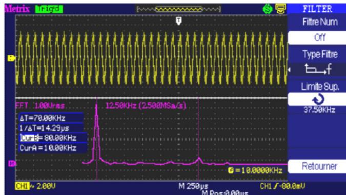
FFT of the signal with the low pass digital filter having a cut-off frequency of 37.5 kHz.
