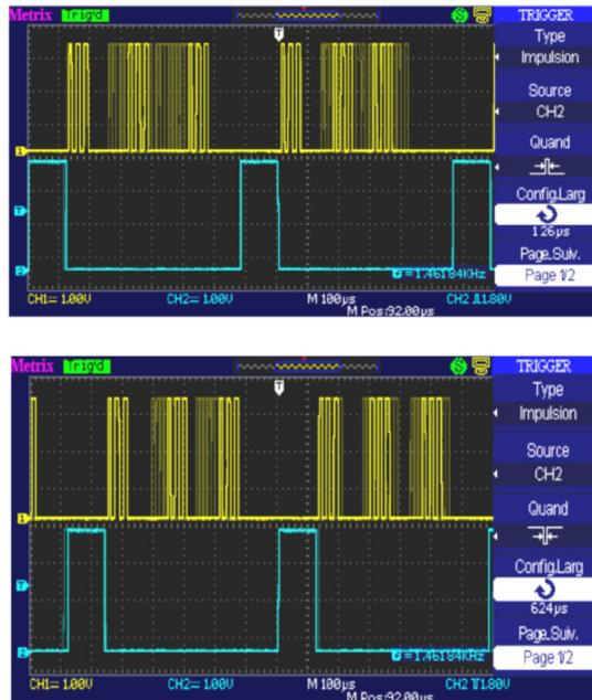
c) Observe the first data group after the negative-going edge of the chip select using the “Delayed” function.
