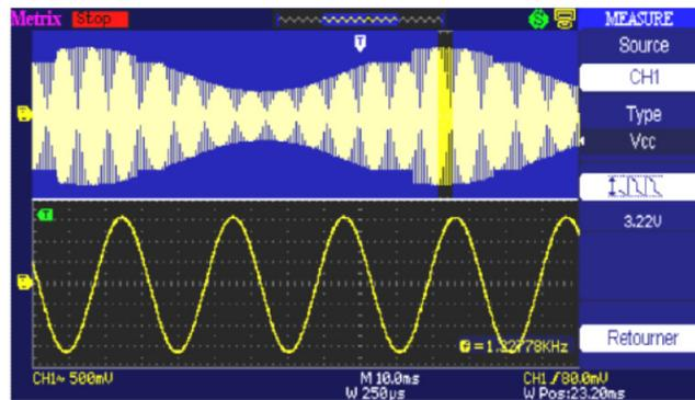
Adjust the oscilloscope so as to display the signals correctly (possible using “Autoset” function).
