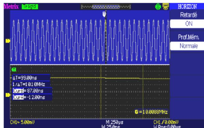
**Conclusion :** By switching the memory depth from “Normal” to “LongMem”, we can record the same time interval with a recording interval 20 times as fine, making possible a finer analysis of the signal, in “Delayed” mode, for example.
