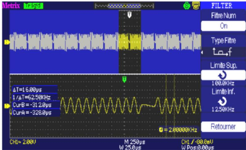
e) A "band-stop" digital filter (25 kHz to 800 kHz) is applied:
