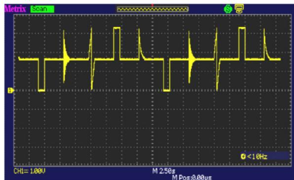
Using triggering on pulse width and acting on the position of the level, it will be possible to trigger on each of the 5 slow signals.
