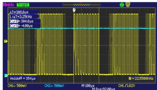
This value must be greater than the duration of the pulse train, to disable triggering during this period, but must remain shorter than the time between 2 pulse trains (which varies between 400 and 480 μs). In our case, the "Hold-Off" must be between 300 and 400 μs.
