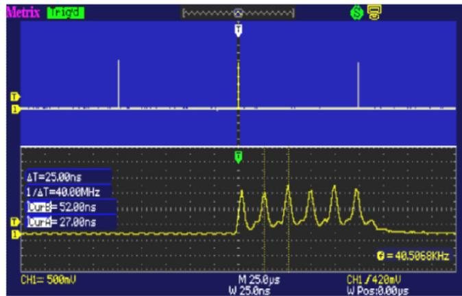
Because of the very brief duration of the pulse (25 ns) compared to their repetition interval (≈ 125 μs), we need a ratio of 1000 between the main time base and the “**Delayed**” time base.
