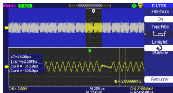
d) A "band-pass" digital filter having a pass band from 12.5 kHz to 100 kHz is applied:
