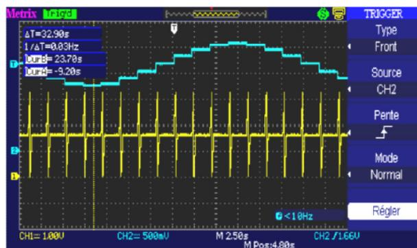
b) Display of Signal no. 13 by Zooming in "STOP", serves to observe one period of signal CH2 and signal CH1 in detail.
