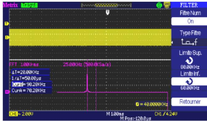
We view the filtered signal and use the cursors to measure its frequency,  $F = 70 \text{ kHz}$  and its amplitude =  $5.12 \text{ V}$  peak to peak:
