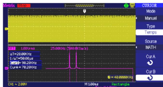
We use a bandpass digital filter (60 kHz 80 kHz) to isolate the 70 kHz spectral spike:
