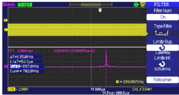
Display of the 900 kHz component with delayed time base:
