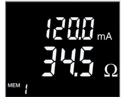
Standard mode: Impedance and leakage current
