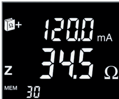
Screen 1: Impedance and leakage current
