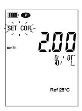
Press the **SET** key and choose the reference temperature (20 or 25°C) using the ▲ and ▼ keys.
