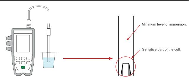
The cell provided with the instrument has an integrated temperature sensor. There is therefore no need to measure the temperature ature of the solution.
