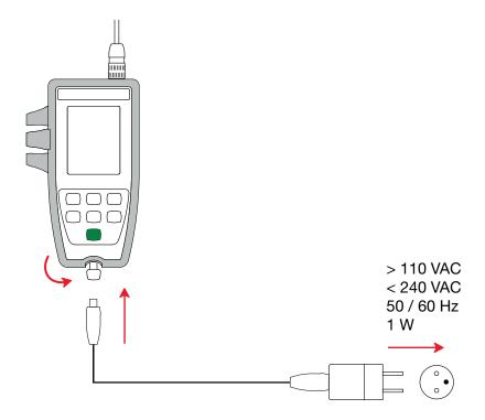
Connecting the external USB supply does not recharge the storage batteries.
