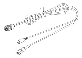
One adapter DIN male to BNC female (for the cell) and female jack (for a PT1000 temperature probe). The cable is 10cm long.
