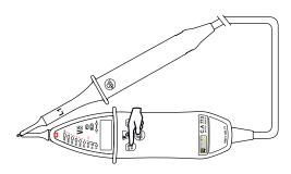
If all indicators on the device except ELV light up, the buzzer sounds and the digital display indicates "ready", the device is operating properly and is usable.
