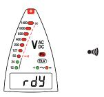
If every second indicator lights up along with the symbol, the batteries must be replaced (see § 5.2).
