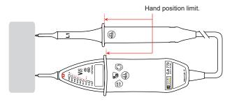
Place the test probes on the element to be tested, and hold them firmly in contact.
