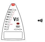
Note: The fact that the Ph indicator is not flashing does not mean that there is not a hazardous voltage on the connector.
