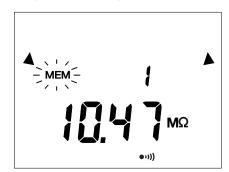
It is recorded with all information tied to it but not necessarily displayed at the time of storage: voltage, current, duration of tests T1 and T2 in the case of PI and DAR, etc.
