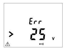
Before the insulation measurement, the instrument is in voltage measurement mode. If there is a voltage on the terminals in excess of 25 V and you try even so to make a measurement, the instrument reports the situation.
