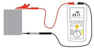
The instrument displays the voltage on the terminals. It detects whether the voltage is AC or DC and, if it is AC, displays its frequency (on the CA 6524 and the CA 6526).
