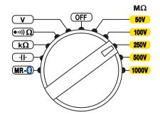
Set the switch to one of the  $M\Omega$  positions.
