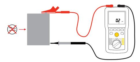
Press the **TEST** button and hold it down until the measurement displayed is stable.
