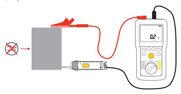
When the probe is connected, the **◄ા** symbol is displayed.
