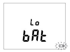
The batteries must then be replaced (see § 5.2), since the battery life indication is no longer reliable.
