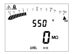
If the measured value is less than the stored value, the display becomes negative.
