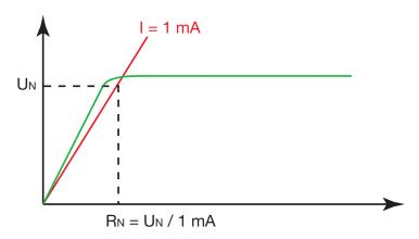
The range of operation per IEC 61557 is from 100k $\Omega$  to 2 G $\Omega$  (see § 4.4).
