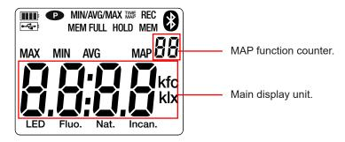
When the measurement exceeds the limit, the instrument displays OL.
