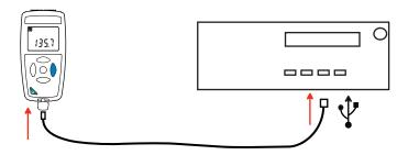
It is treated as a USB key and you can access its content. But to read the records, you must use the Data Logger Transfer software.
