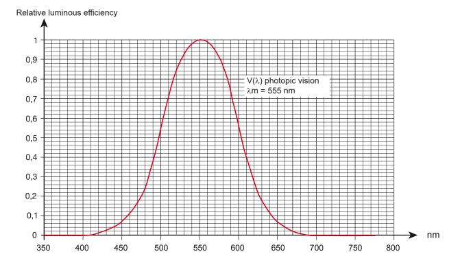
The error on the spectral response of the sensor is equal to the area of the differences between the  $V(\lambda)$  curve and the curve of the sensor.
