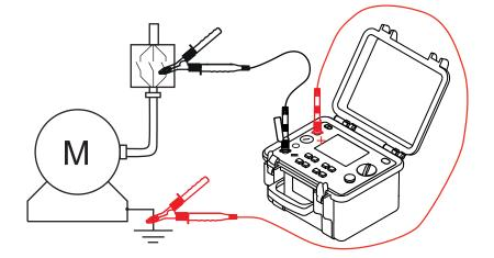
To measure high insulation values (> 1 G $\Omega$ ), we recommend using guard terminal "G" to avoid leakage and capacitive effects or eliminate the influence of surface leakage currents. The guard terminal is connected to a surface where leakage currents may flow through dust and humidity, e.g. the insulation surface of a cable or transformer, between two measurement points.
