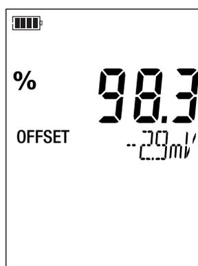
**i** During the calibrations, the slope and offset of a given electrode must not vary more than a little. If you observe a large variation, redo the calibration. If the problem persists, check the buffer solution (in particular the use-by dates) or replace the electrode.
