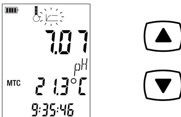
You must then correct the temperature displayed, using the  $\blacktriangle$  and  $\blacktriangledown$  keys, so that it is equal to the measured temperature of the solution.
