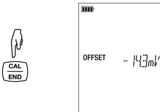
**i** During the calibrations, the offset of a given electrode must not vary more than a little. If you observe a large variation, redo the calibration. If the problem persists, check the buffer solution (in particular the use-by dates) or replace the electrode.
