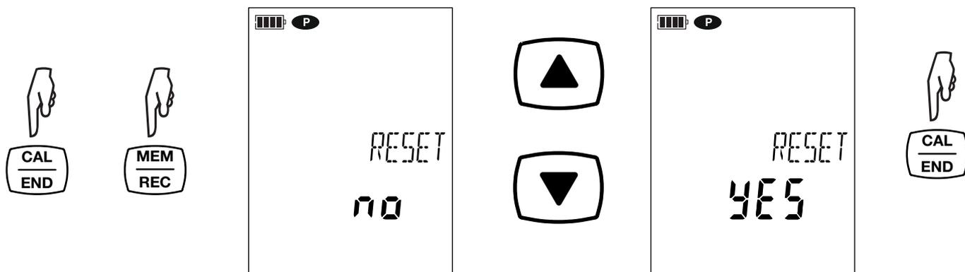
If you do not want to restore the initial calibration, choose **no** (using the **▲** and **▼** keys) before pressing the **CAL** key.
