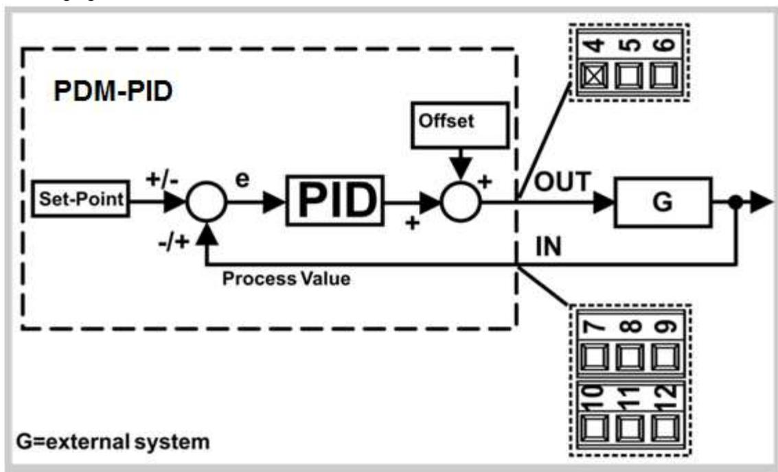
In particular, "e" means the difference between set-point and process-value:
