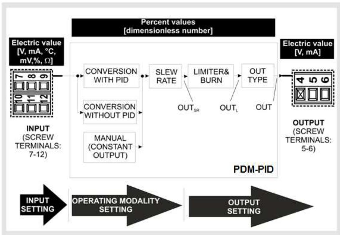
In particular, there are three operating modalities, each of them allows to supply a ON/OFF output or an analog output:
