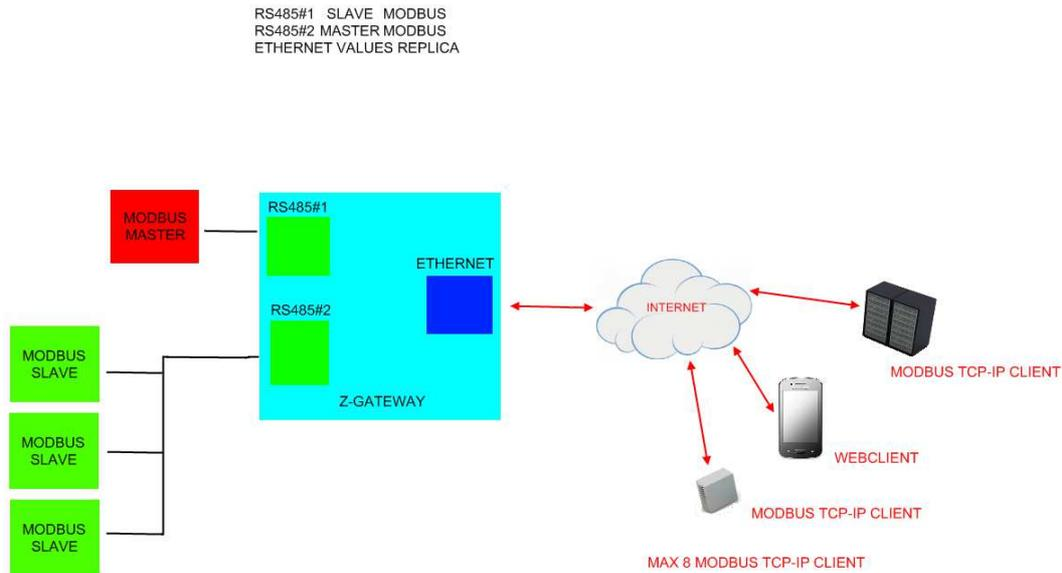
**Shared Memory: RS485#1 and RS485#2 Modbus RTU Slave, Ethernet Modbus TCP-IP server (200 Modbus Registers that can be written and read from a Modbus RTU Master or Ethernet Modbus TCP-IP server, for example:**
