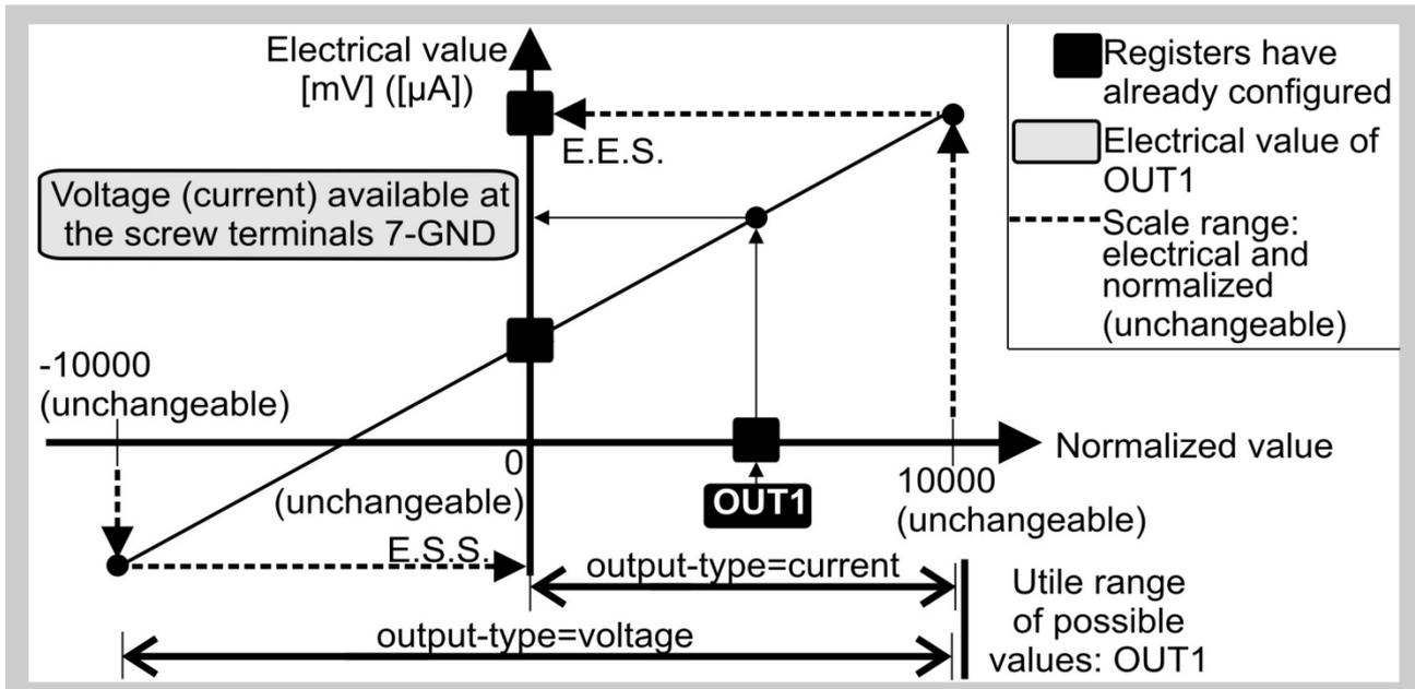
Fig.2 - Description of output configuration (step 3)
