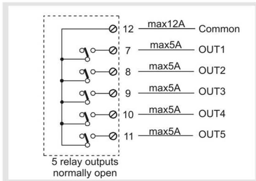
It's forbidden that the current through the screw terminal 12 (common) is greater than 12A. It's forbidden that the current through the screw terminals 7,8,9,10,11 is greater than 5A.
